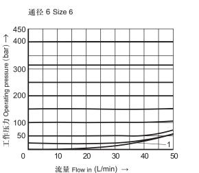
1 = 最低可调压力 1 = Min adjustable pressure
